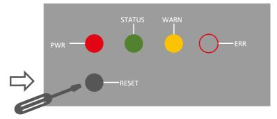
2) As soon as the ERROR LED lights up (approx. 10 seconds after switching on), release the RESET key:
