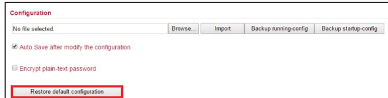
The screenshot shows the 'Config Management' page. At the top, there is a file selection area with 'No file selected.' and buttons for 'Browse...', 'Import', 'Backup running-config', and 'Backup startup-config'. Below this is a configuration section with two checkboxes: 'Auto Save after modify the configuration' (checked) and 'Encrypt plain-text password' (unchecked). At the bottom of the configuration section is a red-bordered button labeled 'Restore default configuration'.
